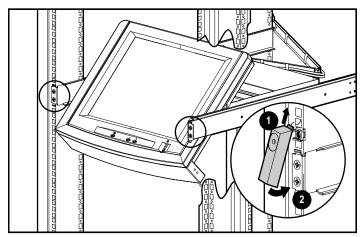
Figure 2-7. Attaching the retma rail covers
